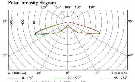
$0^{\circ}$  Imax= 315 cd/1000lm for C=275° and  $\gamma$ =70°
